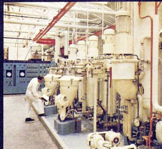
Below: This new continuous-process soap making plant by De Laval is the first complete installation of its kind in this country.
